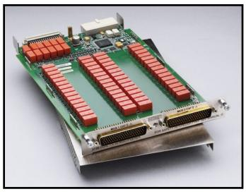
The Model 3720 offers two independent banks of 1×30 two-pole multiplexers. It is ideal for general purpose switching, including temperature measurements. The two banks can automatically be connected to the Series 3700A mainframe backplane and optional DMM through the analog backplane connection relays. This connection allows the mainframe to reconfigure the card to a single  $1 \times 60$ two-pole multiplexer or to enable card-to-card expansion for even larger configurations.
